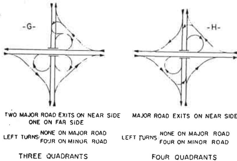
Schematic of partial cloverleaf ramp arrangements, exit and entrance turns.
