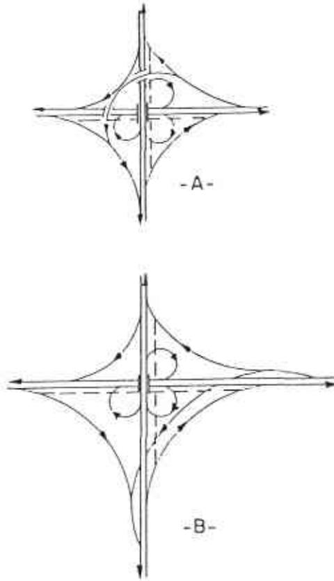
NOTE: WEAVING ADJACENT TO THE THROUGH LANES IS ELIMINATED BY PROVIDING COLLECTOR-DISTRIBUTOR ROADS AS SHOWN BY DOTTED LINES.
